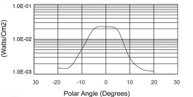
**Radiant Exitance (Watts/Cm2):** Volts = 1.50, Distance = 3.0 inches from source
